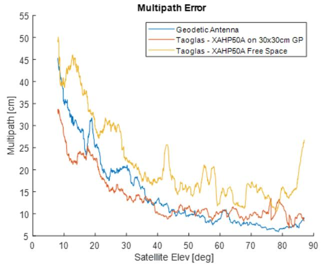
Fig. 7. Standard deviation of the multipath error for GPS L1-C/A signal.
