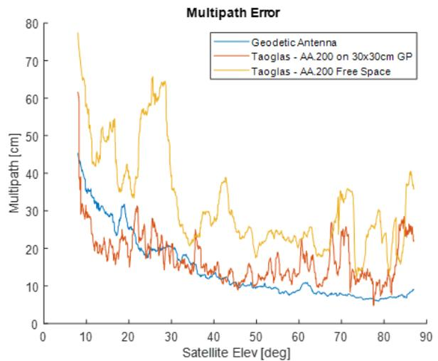
Fig. 8. Standard deviation of the multipath error for GPS L1-C/A signal.
