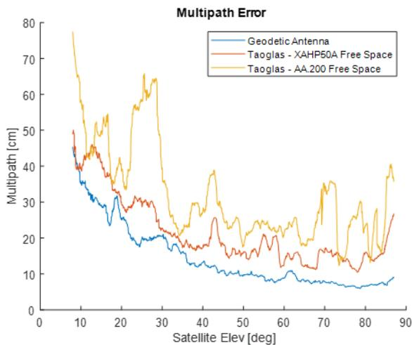
Fig. 6. Standard deviation of the multipath error for GPS L1-C/A signal.
